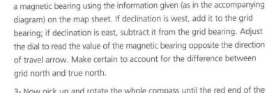
3. Now pick up and rotate the whole compass until the red end of the needle points to the north marker on the dial. The direction-of-travel arrow on the compass card will point to your destination. Choose a landmark in that direction and walk towards it.
