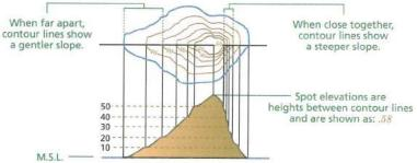
Contour lines connect a series of points of equal elevation and are used to illustrate relief on a map. They show the height of ground above Mean Sea Level (M.S.L.) in either feet or metres and can be drawn at any desired interval. For example, numerous contour lines that are close to one another show hilly or mountainous terrain; when far apart, they indicate a gentler slope.
